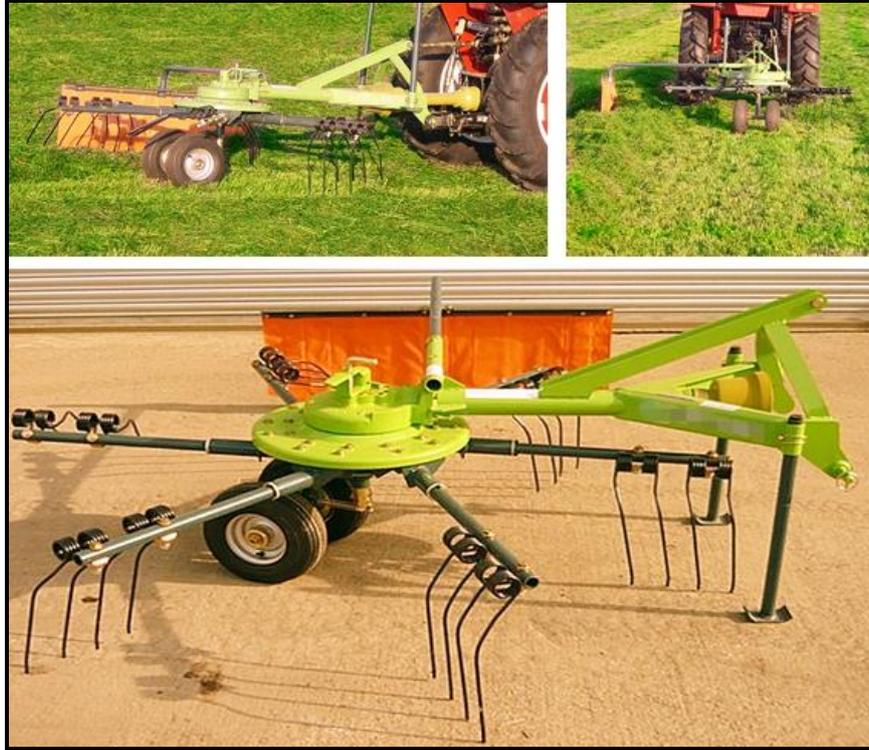
Ideal for rowing up before baling fully will also spread freshly mown grass to aid with fast drying
