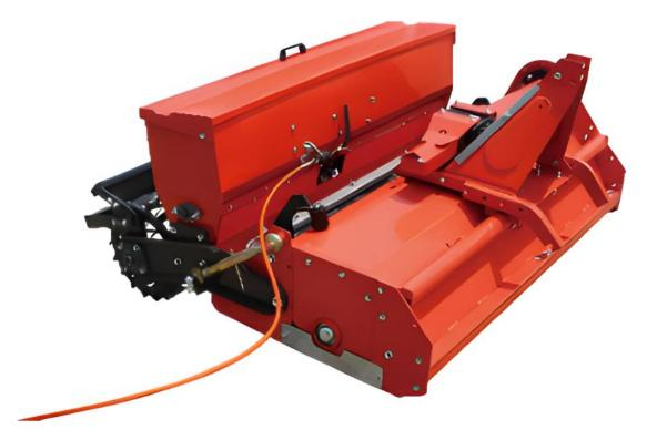
The Siromer stone burier cultivates, buries stones, levels to prepare the perfect bed. The stones, clods, old turf and debris are centrifugally separated out and thrown to the bottom of the soil profile. A screen gradually releases the renovated material with the finest soil at the top, this then passes under the mesh roller which gently levels off the soil leaving a bed perfect for seeding.
