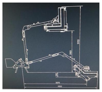
With a 4.5m horizontal reach and 3.7m vertical reach, capable of cutting on top of a 2.5m hedge.
