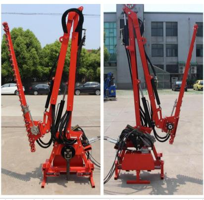
A lightweight hedge trimmer complete with a 1.9m cutting head.
