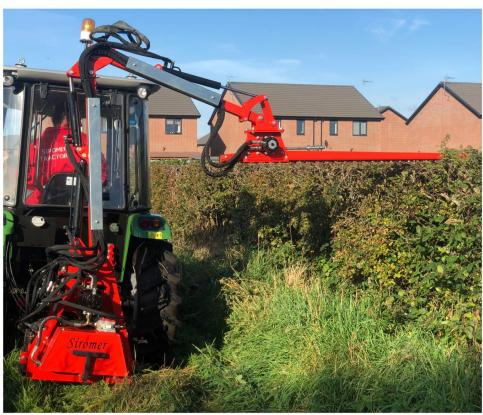
Siromer Hedge Trimmers are designed to fit industry standard CAT I linkages.
