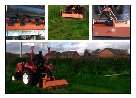
The Siromer Flail Mower is designed for grass cutting in fields, parks or orchards. Available as fixed semi offset or with hydraulic offset. (Double acting spool required for operation of hydraulic side shift.) All flail mowers are fitted with high power gearbox and robust drive line to give hassle free mowing. Complete with a support leg for storage. The fixed semi-offset flail mowers are offset by approximately 6 inches.
