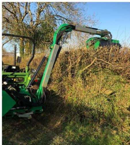
Siromer's high-reach flail hedge trimmers are fitted with a PTO driven hydraulic pump, which means the hedge trimmer is independent of the tractor's hydraulics.
