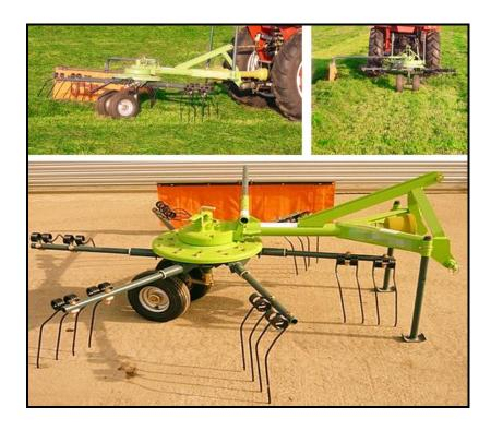
Ideal for rowing up before bailing fully will also spread freshly mown grass to aid with fast drying As a tedder:
