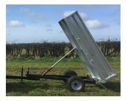
2.5 ton capacity Very high tilt 2.5m (8ft) x 1.5m (5ft) Galvanized body Drop down sides and rear (leaving very useful flat deck). Rear door can be hinged from the top or bottom.
