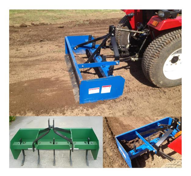
Fitted with a standard CAT I 3-point linkage
